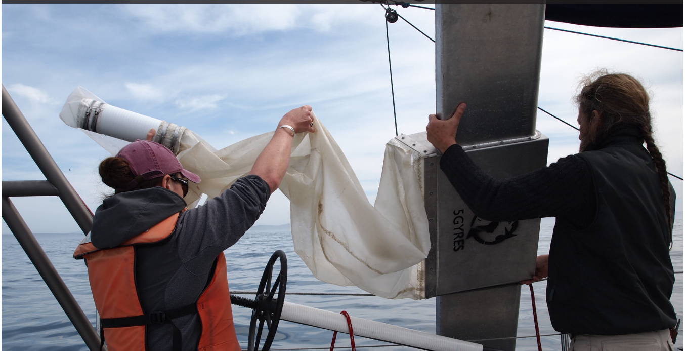
Launching manta trawl during surface water sampling • Photo by Erika Delemarre
