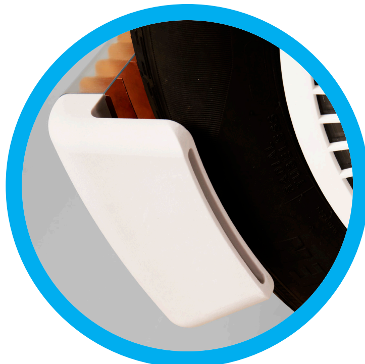
On-vehicle tire debris collection system. Courtesy of The Tyre Collective.
